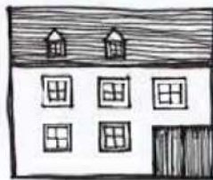
Loft conversion incorporating gabled dormers.
